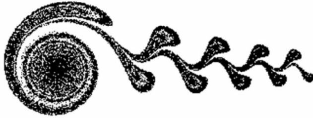
Fig. 2. Von Karman streets simulation (Parameters: b = 0.9, d = 2\pi, a = 1, k = 4, t = 10 )
